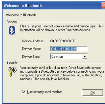
After finishing the setup, click <confirm> to enter the main window of IVT software. If want to search Bluetooth equipments, please confirm Bluetooth function of other Bluetooth equipments start (some kind mobile phones need to setup their visibility), then click the ball button in the main window of IVT software to search. If finding any equipment, the name of these equipments will be showed in the orbit near to the ball. Here take phone communication for example:
