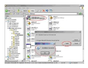
3 \ Use USB cord to connect G-RAYS 2 to the USB port of computer. Computer will automatically check it and seek driver software by itself. If PC asks for "device manager" for adding the new USB device following USB device connection, take the procedure below. Click "next".
