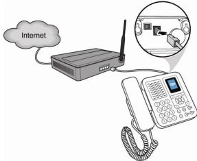
4. Connect one end of the power adapter to the phone's power jack. Plug the power adapter into a mains outlet.
