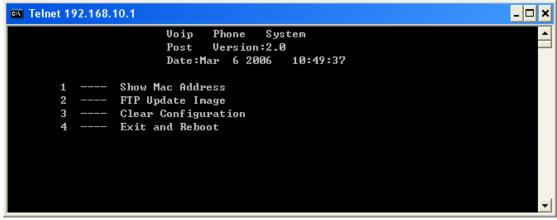
IP521 provide safe mode. When there is booting problem because of setting problem or firmware problem. User can restore the factory setting or upgrade to a new firmware to solve this problem.
