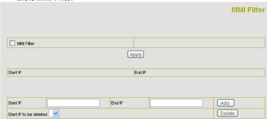
MMI filter is used to make access limit to IP521 IP phone. When MMI filter is enable. Only IP address within the *start IP* and *end IP* can access IP521 IP phone.
