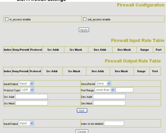
Firewall setting page. User may set up firewall to prevent unauthorized Internet users from accessing private networks connected to the Internet (input rule), or prevent unauthorized private network devices to access the internet.
