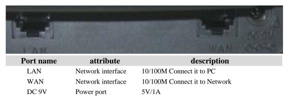
FV6030 is provided with two Ethernet cables and a power adaptor. Phone has two interfaces: WAN and LAN. Please refer to safety notes of this manual carefully before power adaptor is connected.
