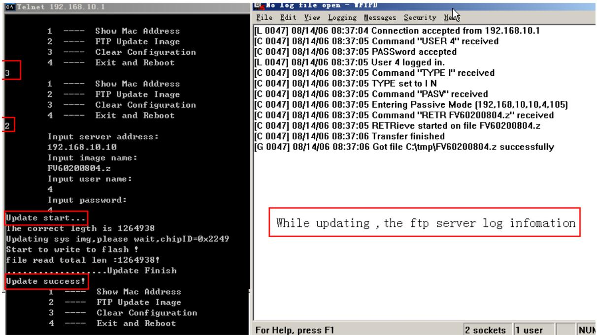
The phone provide safe mode. When there is booting problem because of setting problem or firmware problem. User can restore the factory setting or upgrade to a new firmware to solve this problem.
