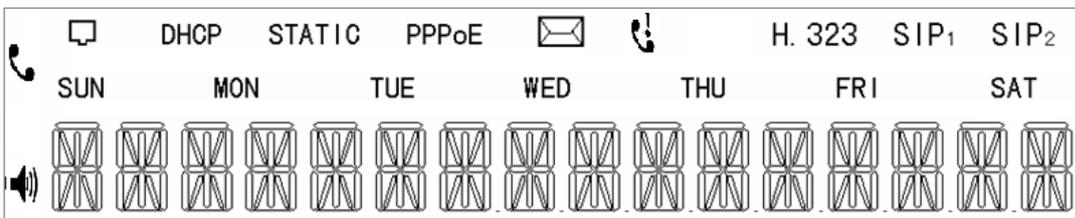
The LCD is equipped with a backlight. When the phone is in the normal idle state, the backlight is off. Whenever an event occurs, the backlight turns on automatically and brings the user's attention. The definitions for each character displayed on LCD described as below table.
