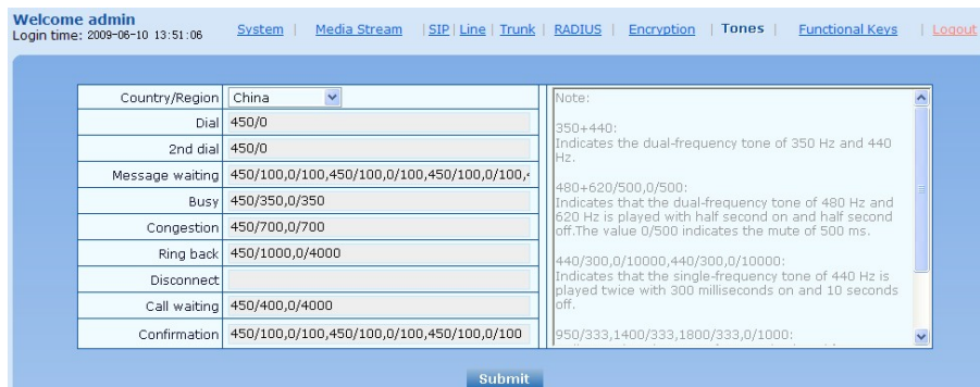
Figure 2-19 Call progress tone configuration interface
